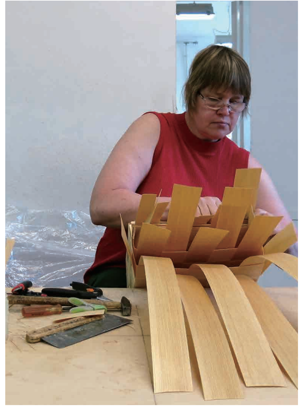
非常に薄いスプリントやベニヤは割れたり裂けたりしやすいため、かごを編む前に軽く水に漬けて柔らかくし、丁寧に扱います。 Splints and veneers are still thin pieces of wood that could split or break if not handled correctly when weaving. They are lightly softened with water before weaving.
