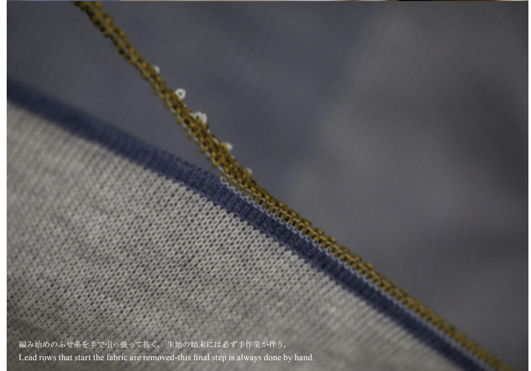
編地と編地をつなぎ合わせる、リンキング作業。 Separate pieces of knitted fabric are joined together in the linking process.
