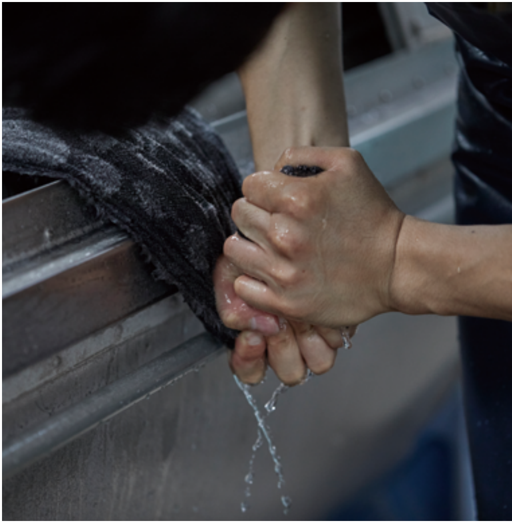
縮絨後の生地を絞る作業。素材や色によって縮み具合はそれぞれ。生地によって湯の温度や洗う時間を微調整して縮絨する。 The degree of fulling varies depending on the material and colour. During this process, water temperature and washing time are finely adjusted to the particular fabric. The fabric is then fulling and wrung out by hand.
