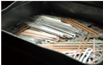
経糸が切れた時に知らせてくれるパーツ、ドロッパー。 'Droppers' are used to show where the warp has been cut.
