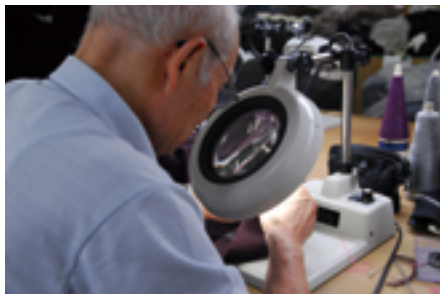
編み機が落とした編み目を丁寧に拾う。 An expert knitter carefully picks up a stitch dropped by the knitting machine.
