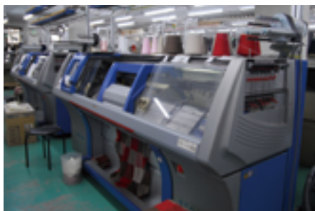
商品をつくるのに最適なスピードで編み機が動く。 Knitting machines for each item are adjusted to operate at the optimal speed.
