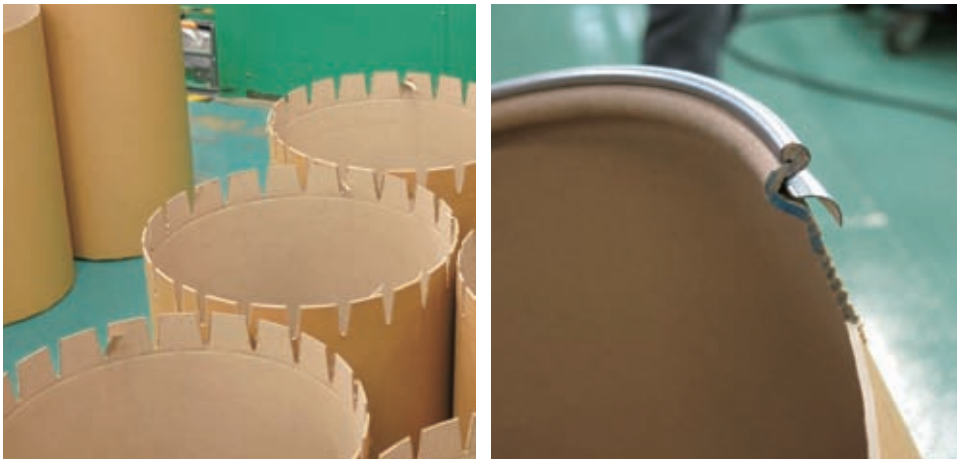
(左) 紙に切り込みを入れて折り返しを作り、内側に折り曲げて底板に接着します。 (L) Shapes are cut into the paper to create flaps, which then are folded and glued onto the base component. (右) エッジ断面。金属で強化されています。 (R) A sectional cut of the rim showing the metal reinforcement.
