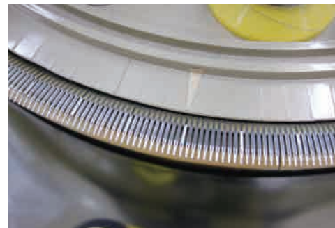
編地と編地をつなぎ合わせる、リンキング作業。 Separate pieces of knitted fabric are joined together in the linking process.
