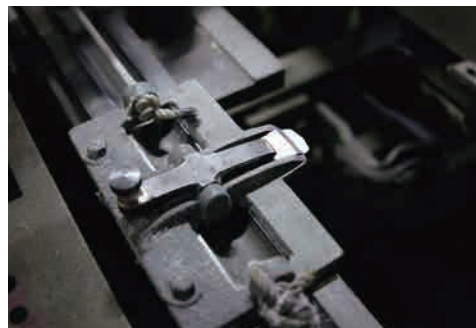
織機と一体になった刃。カットと研磨を同時に行う。 An integral part of the loom, this cutter performs both cutting and grinding simultaneously.
